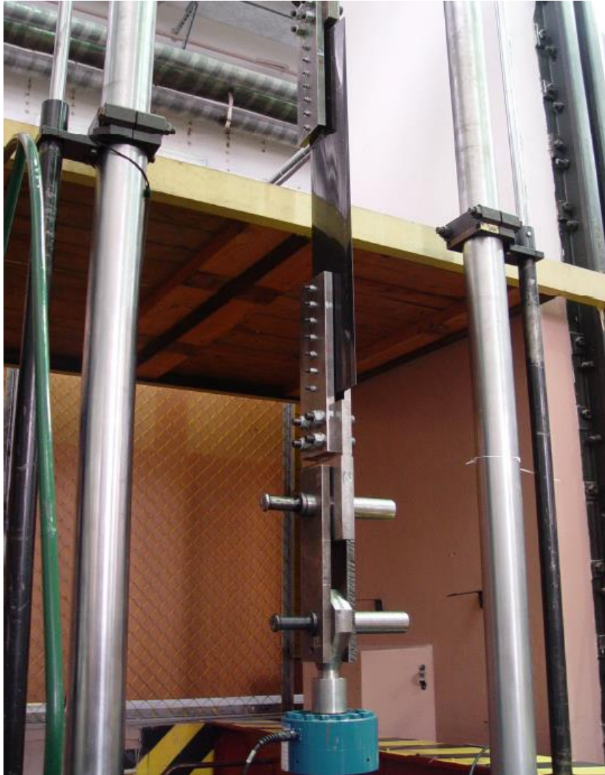
Fig. 1. The tested blade fragment mounted on the testing station.
