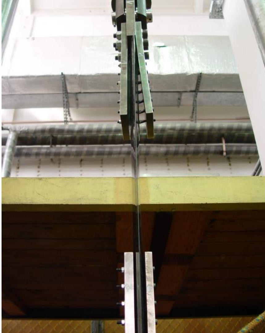
Fig. 2. The destroyed bolts connection in the tested element on the testing station.
