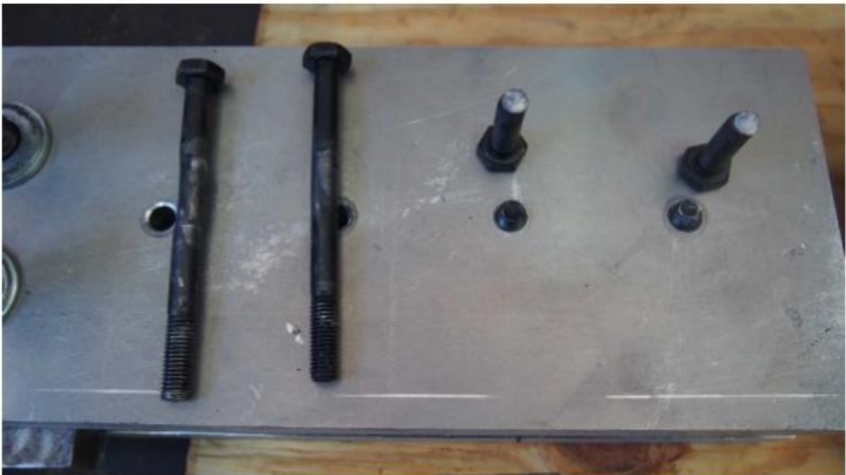
Pic. 4. Destroyed bolts connection of the blade with the handle (after disassembly)
